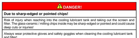
The cooling lubricant tank must be emptied and cleaned every two weeks. Always dispose of cooling lubricant residues in accordance with the legal provisions and local regulations!
